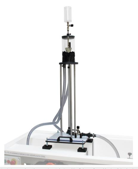
The goal for this apparatus is to reproduce the experiment designed by Osborne Reynolds visualizing laminar, transitional and turbulent flows, and establishing the Reynolds number that corresponds to each one of them.
